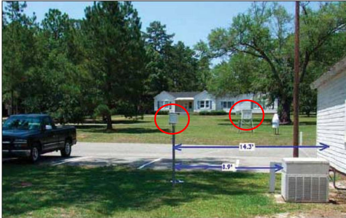
Figure 15. Old Stevenson Screen and new MMTS/Nimbus electronic thermometer in Bainbridge, Georgia. The new station is recording heat from the air conditioning unit, house, cars, and asphalt parking lot. Shading issues mean winter temperatures are also affected when leaves are absent.
